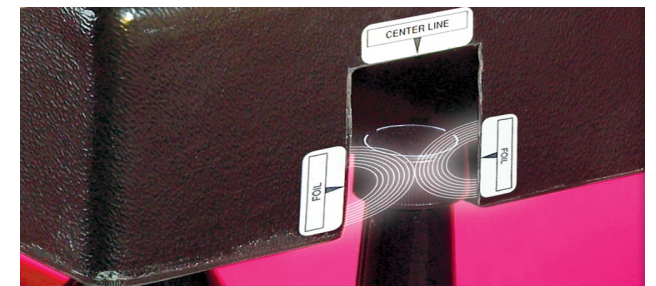
DEEP TUNNEL SEALING HEAD
