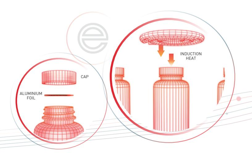
The induction coil delivers a controlled electromagnetic field that transfers energy to the foil instantaneously creating heat.
